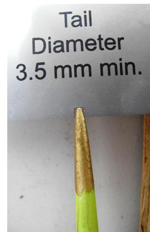
*This jav's tail was "sharpened" and then painted over. However, it fits within a 3.5 mm notch. It should be repaired or disqualified*
